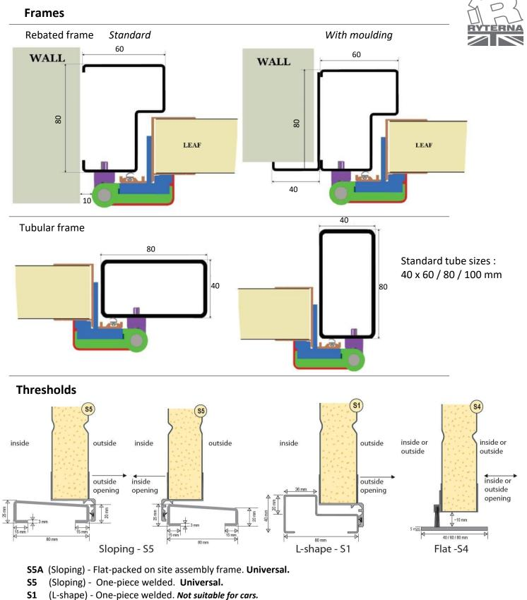
S4 (Flat) - One-piece welded. Water penetration is likely.
